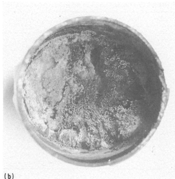
Figure 2 (a) Schematic drawing of the cross-section through a crucible, and (b, c) enlarged photos of crystal groups with diameters about 0.2 mm at 500 °C.
